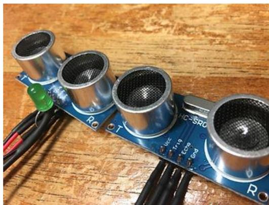
*Figure 4 - Wiring of Ultrasonic sensor and LED.*
