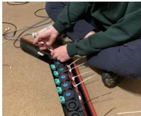
*Figure 10 - Wire management on the vent-visor assembly.*
