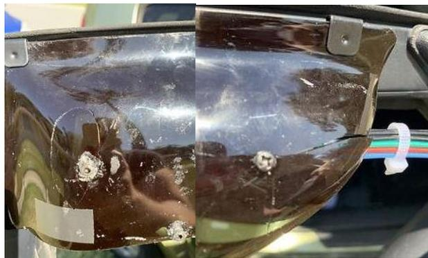
*Figure 11 - Breaks in the vent-visors.*
