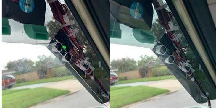
*Figure 9 - The Green LED is on when the window is down and off when the window is up.*
