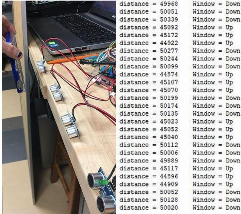
*Figure 6 - Testing integrated operation of all four ultrasonic proximity sensors.*
