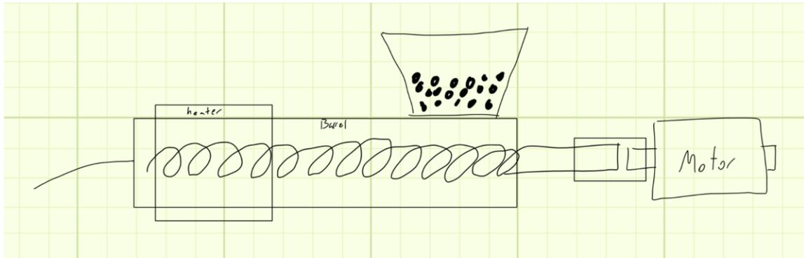
Figure 2. Design Concept A. "Screw Auger" motion. The raw material is moved through the extruder barrel by a screw auger i.e. an auger style drill bit turned in reverse. This is sized to be a close fit to the size of the barrel such that the pellet material is forced forward with the motion of the screw. The power comes from an electric motor coupled to the screw, possibly with a gear reduction. This sketch was drawn by Vincent Mazzochette on September 27th 2023.
