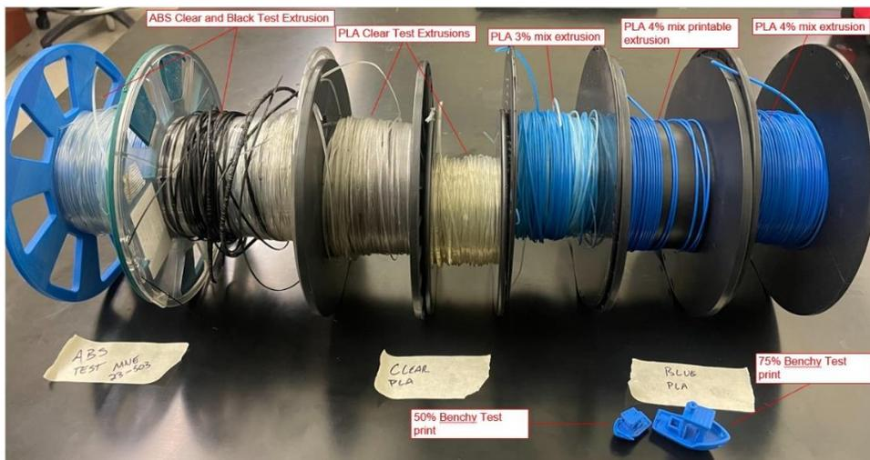
Figure 9. Testing spools fabricated using the modified Lyman Extruder
