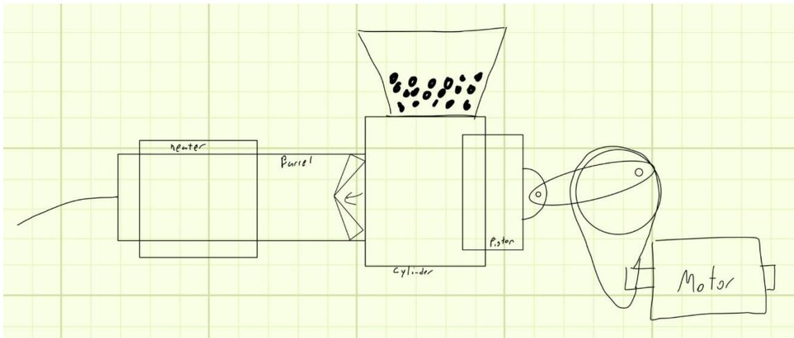
Figure 3. Design Concept B. "Piston Pump" motion. The raw material is moved through the extruder barrel by a reciprocating piston pump. The reciprocal motion of the pump is negated within the material by way of a one way valve within the barrel. The power comes from an electric motor coupled to the piston by way of a set of pulleys and a crank rocker. This sketch was drawn by Vincent Mazzochette on September 27th 2023.
