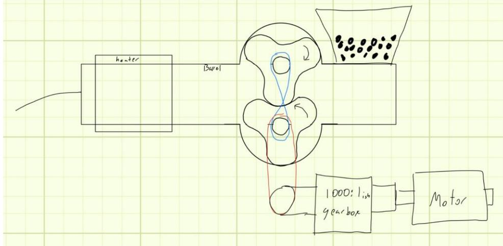
Figure 4. Design Concept C. “Vane Pump” motion. The raw material is moved through the extruder barrel by a vane pump, similar to that of an air compressor or supercharger. The power comes from an electric motor coupled to the piston by way of a set of pulleys and a high ratio gear reduction gearbox providing very low RPM but high torque to the pump. This sketch was drawn by Vincent Mazzochette on September 27th 2023.
