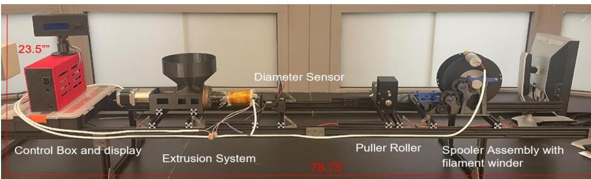
*Figure 1. Physical Prototype Extruder. The team envisions a fully mounted extruder system that allows independent adjustments in the X, Y, and Z axes for optimal precision and versatility.*
